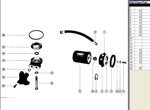
ACCESSORIES (Instruments-Gauges and Components) Serial Nbr Range: MC Misc. (1985 and Below)
